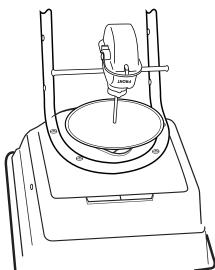
**4.** Install gearbox by inserting the pinion shaft into hole in center of hoppers bottom. The word "FRONT" on the gearbox must point to *Front* of the hopper. The EarthWay logo is on the front of the hopper.
