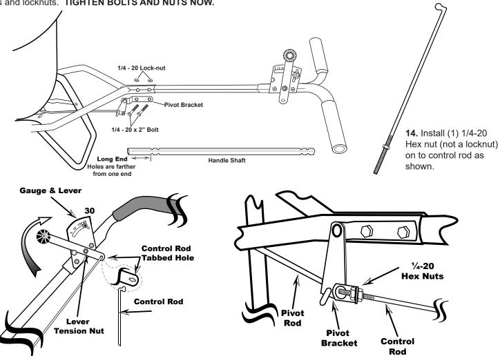
**15.** Install flattened end of control rod in to lever on gauge as shown. Turn to lock in place. Next push lever forward to setting "0". Align control rod with hole in pivot bracket, pull lever backward to insert control rod through hole in pivot bracket. Now install 1/4-20 Hex nut on to control rod.
