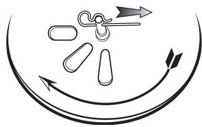
**18.** Insert agitator to pinion shaft on inside of hopper. **Note:** the position of flat side of the agitator. This pin should be installed as shown.
