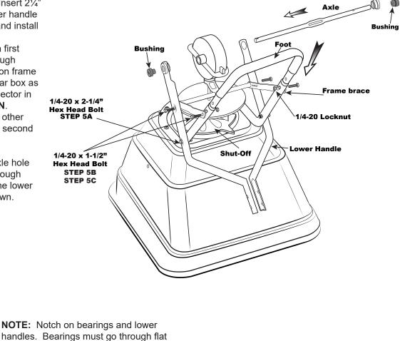
NOW GO BACK AND TIGHTEN ALL NUTS AND BOLTS STARTING WITH FIRST STEP. <u>DO NOT OVER TIGHTEN.</u>
