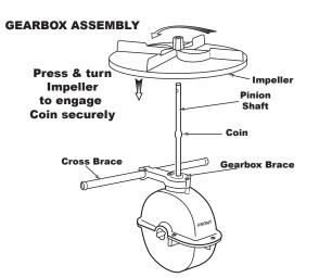
**3.** Install impeller onto pinion shaft by pressing the impeller as shown onto the pinion shaft and turning the impeller while holding the pinion shaft to engage with the *COIN* fully, and press down to secure.
