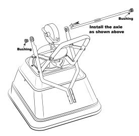
7. Slide axle bushing over axle and into axle bearing to both sides as shown.
