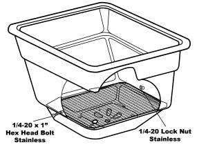
**19.** Install debris screen into hopper, then insert 1/4-20 x 1" Stainless Steel Hex Bolt thru the hole in the side wall of the hopper. Secure with Stainless Steel lock nut - **TIGHTEN WITH HAND TOOLS ONLY**
